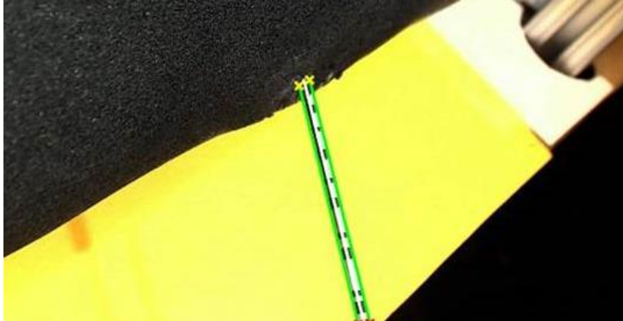
Figure 17 - The results of the Hough transform line detection on the left image show the wire edges outlined in green.
