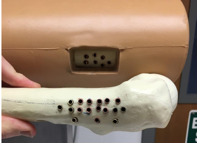
Figure 29 - The target sawbones are pictured here. The target slots are shown to cover the workspace provided in the window of the soft tissue envelope.
